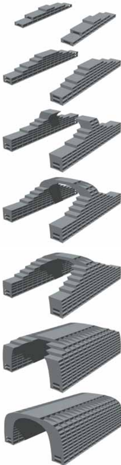
The structural engineers for the arched structure, DHV B.V., of Rotterdam, refer to the construction technique that will be used to build the arch in two directions, with individual units of floor and wall extending toward each other, as the kissing act.
